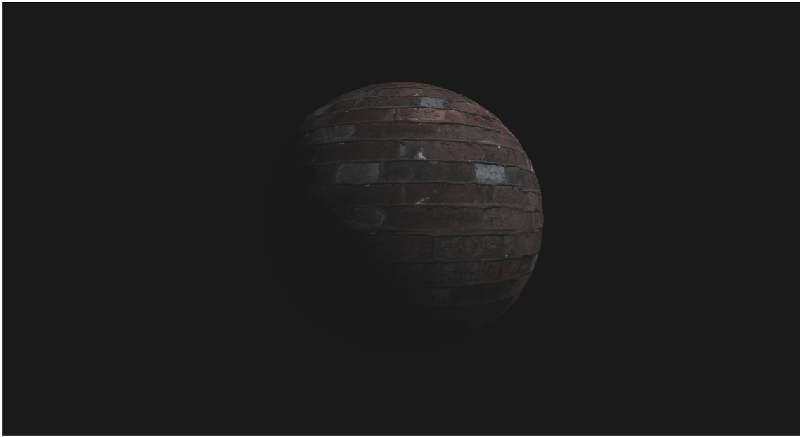
Figure 3: Same Phong BRDF material with a normal map. Renderer can be found at https://github.com/torresguilherme/bits-of-opengl
